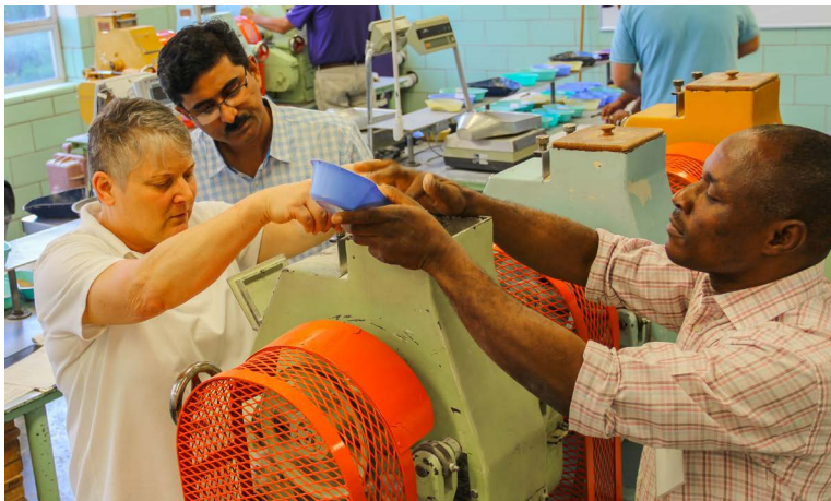
Shellenberger Milling Laboratory – table-top milling equipment provides a hands-on understanding of the basic grinding techniques used in the flour milling process
